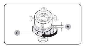
3. Hold the adaptor and turn part (C) in the arrow direction to loosen it by 5 mm (\*).
