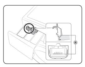
First insert the provided liquid container in the II main-wash compartment. Then, apply liquid detergent to the container below the marked max line (A).
