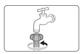
**7.** If using a screw type of water tap, connect the water hose to the water tap as shown.
