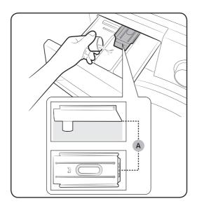
**3.** Apply fabric softener to the **softener** compartment. Do not exceed the max line (A).
